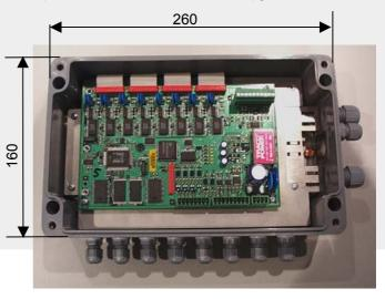
Housing height: 90 mm Fixing screw spacing: 240 x 110 mm fastening material is supplied.
